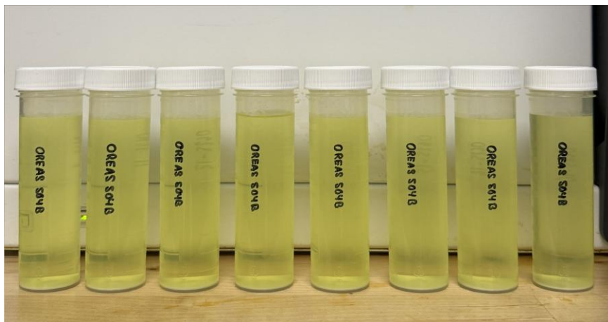
Figure 1. OREAS 504b digestates following ColdBlock aqua regia digestion, prior to ICP/ICP-MS analysis.
