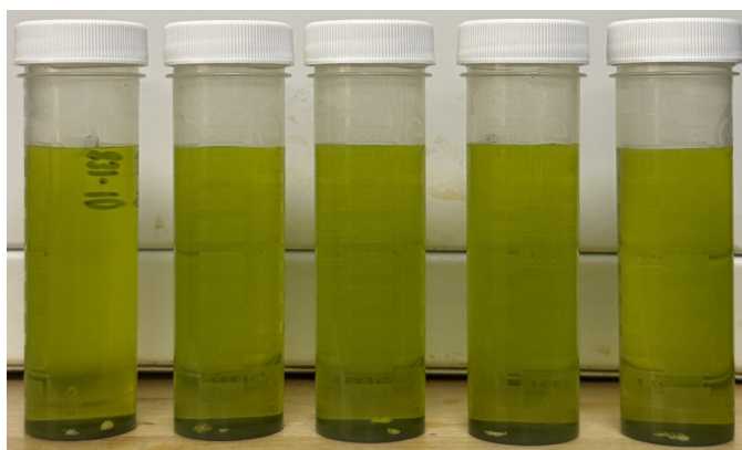
Figure 1. BAM-M505a digestates following ColdBlock HNO 3 /HCl digestion (Method 1).
