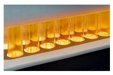
ColdBlock's aqua regia digestion methods for Gold analysis take less than 20 minutes, and ColdBlock digesters can accommodate samples sizes up to
